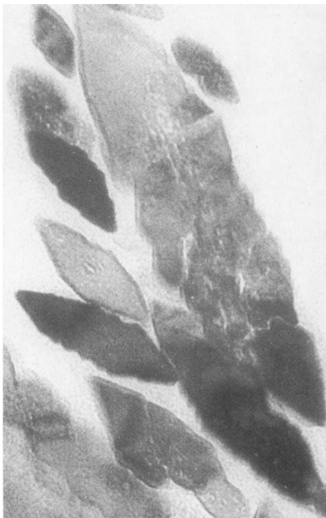
Fig. 5-3. High resolution electron micrograph of a thin section of acicular goethite crystals cut perpendicular to the crystallographic b-direction (needle axis). The lattice images (ca. 1 nm) seen in one crystal correspond to the a-dimension of the unit cell (0.9956 nm). The crystals are bounded by (101) faces. (Schwertmann, 1984; with permission). (Courtesy H. Vali).
